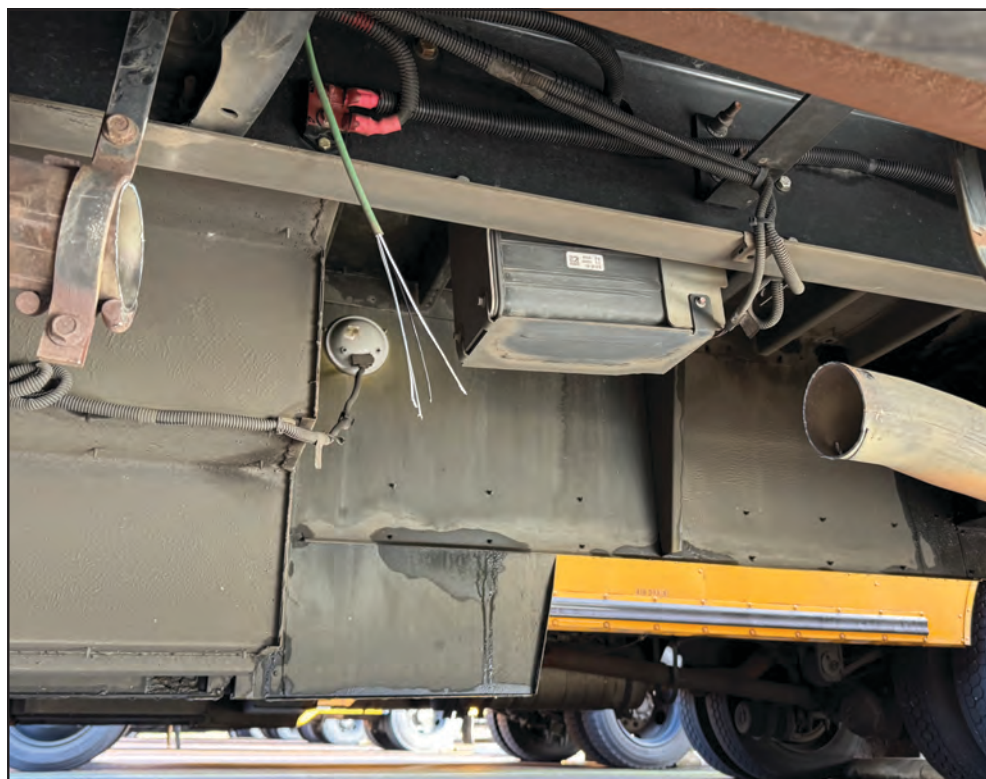
Photo courtesy of Lebanon Community Schools Sawed-off exhaust pipes, left and right, show damage on a school bus after someone stole the catalytic converter.
